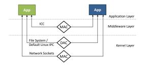
Figure 2: Communication channels and respective access control mechanisms in Android.
