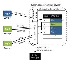
Figure 5: Coloring of data (1) and isolation of data from different colors in the (2) System Content Providers and (3) System Service.
