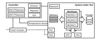
Figure 2: Device and software setup
