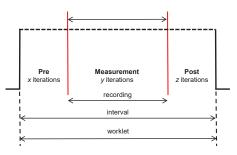
Figure 6: Phases of a Fixed Iteration Sequence
