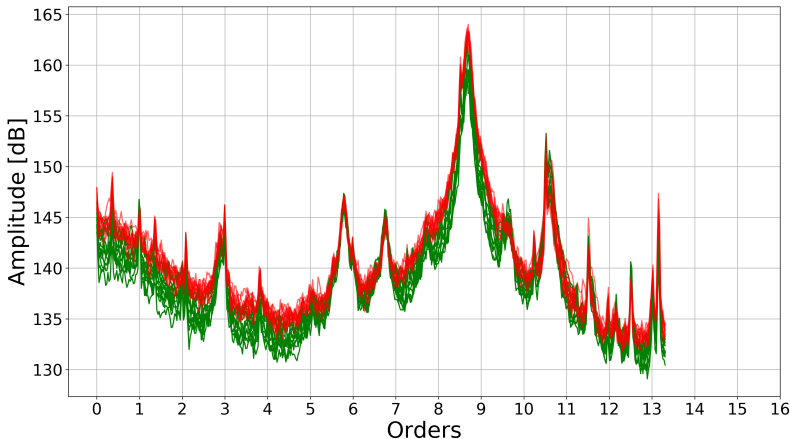
Figure 9.1: Order spectra of all measurements in X direction for the second unbalance phase P5. Measurements of the experiments with attached unbalance are plotted in red, measurements of the normal experiments are plotted in green.
