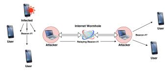
Fig. 7: Wormhole attack setup to relay BLE beacons
