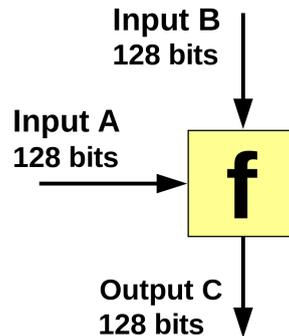
Figure 2.2.: One-way compression function [22]
