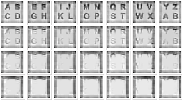
Figure 8: Watermarks after watermark overwriting with eleven keys. The lines correspond to the first four hardening steps with accuracy drops from 89.10% to 83.89%, 70.38%, 56.39%, and 46.52%, and SSIMs of 0.52, 0.17, 0.05, 0.01.
