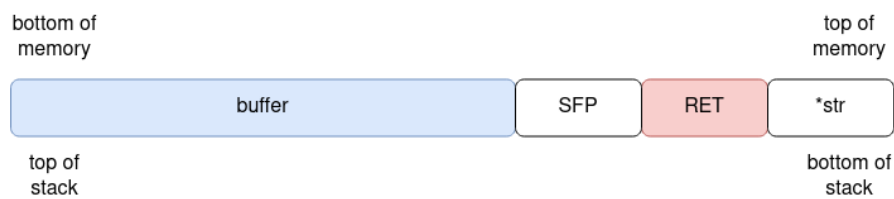
Figure 2.1.: Stack layout when calling “function” [19].
