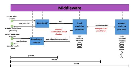
Figure 2: Application example of a CPN in the field of Ambient Assisted Living (Smart Home)
