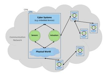
Figure 1: A Cyber-Physical Network containing several Cyber-Physical Systems
