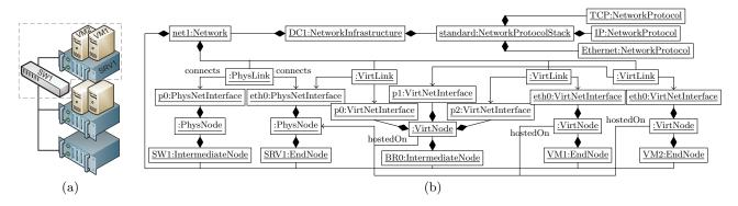
Figure 5: Selected fragment of an exemplary data center network (a) presented on the object diagram (b).
