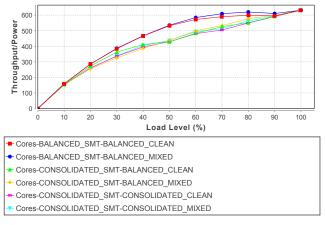
Fig. 16. Energy efficiency of heterogeneous load distribution strategies on Haswell single-socket system.
