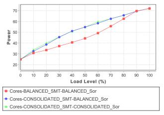
Fig. 2. Power consumption of distributions for SOR on single-socket system.
