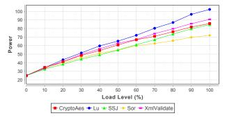
Fig. 4. Power consumption of fully consolidated load on single-socket system.
