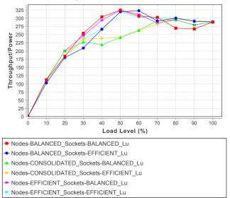
Fig. 14. Energy efficiency of load distribution strategies on two nodes using the Haswell dual-socket system for LU. Unused nodes remain in an idle state.
