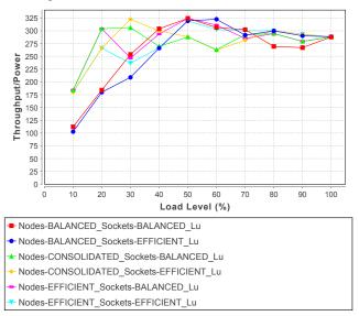
Fig. 13. Energy efficiency of load distribution strategies on two nodes using the Haswell dual-socket system for LU. Unused nodes are turned off.
