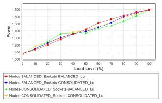
Fig. 15. Power consumption of load distribution strategies on two HP dualsocket nodes for LU. Unused nodes remain in an idle state.
