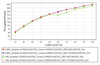
Fig. 6. Energy efficiency of consolidated strategy with and without SMT unit consolidation on both dual-socket systems for SOR.
