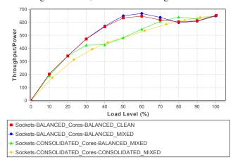
Fig. 17. Energy efficiency of heterogeneous load distribution strategies on Haswell dual-socket system.
