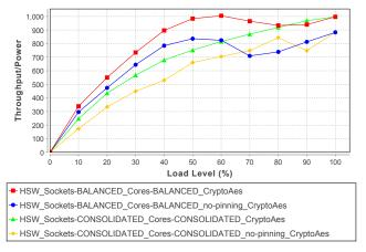
Fig. 11. Energy efficiency of load distribution strategies, including nonpinning strategies, on Haswell dual-socket system for CryptoAES.
